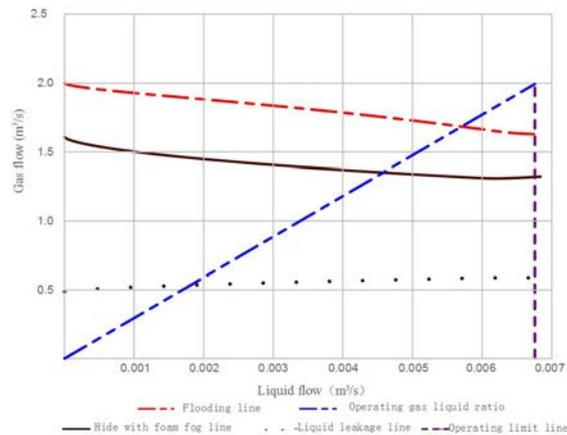
Figure 2: Load performance diagram for the rectifying section.
