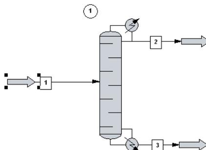
Figure 4: Calculation model - shortcut method.
