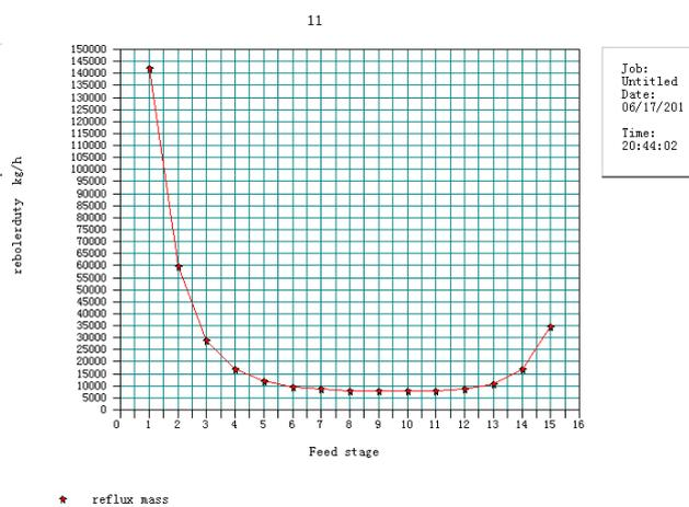
Figure 6: Curve of the return quality change with material plate location.
