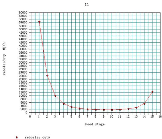
Figure 5: Curve of the reboiler heat load change with material plate location.
